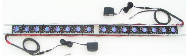
Note that to operate properly, Cool-stick requires a gap of at least 3/4" below and above the panel. Ideally, there should be no gap at either side, so that airflow is strictly from bottom to top.
